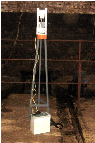
Fig. 3. General view of mobile unit for microclimate parameters measuring
