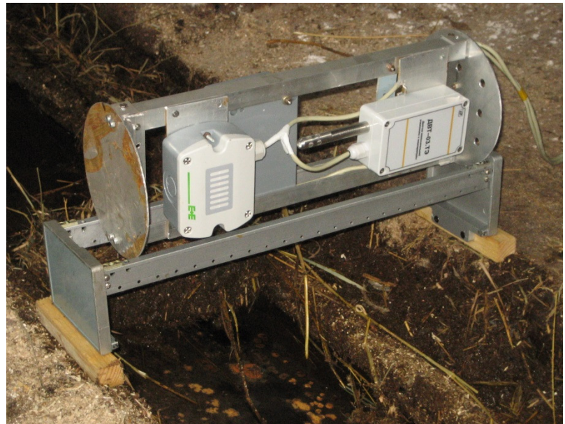
Fig. 4. Measurement of CO 2 concentration in the process of manure removal
